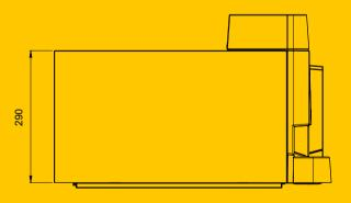
Front space required to fold up the note recycling module: 620 mm
